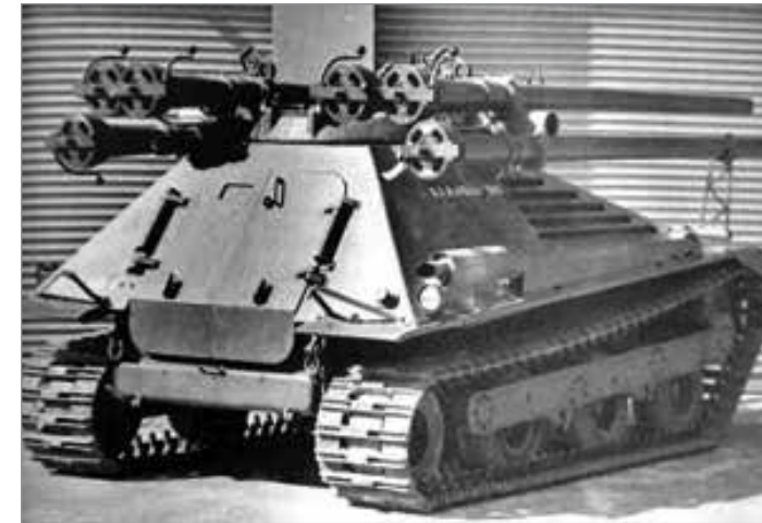
The impressive-looking M50 Ontos tank destroyer held a formidable rifle array which had to be reloaded from the outside of the vehicle.
